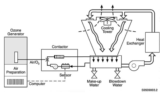
Fig. 2. Process for Ozone Treatment of Cooling Tower Water
