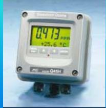
Display Range: 0-200.0 PPB, 0-2.000 PPM Accuracy: ± 0.02 PPM or 0.5% of F.S. Repeatability: ± 0.01 PPM or 0.3% of F.S. Linearity: 0.1% of F.S. Zero Drift: < 0.01 PPM per month Materials of construction that provide excellent to good performance with ozone:
