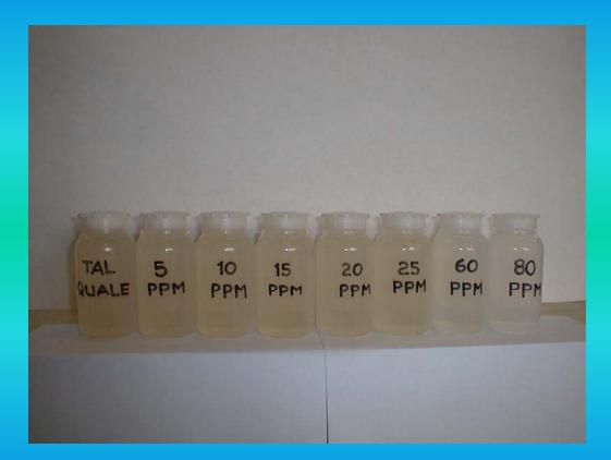
Textile Mill Wastewater Treated with Ozone
