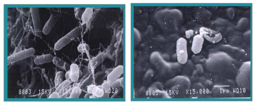
1. Ozone oxidizes cell membrane, causing osmotic bursting
