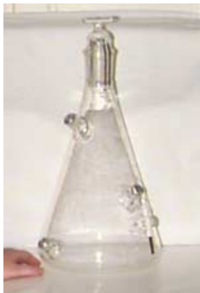
Fig. 4. Photo of the type of reactor used in large batch experiments (4.5 L).
